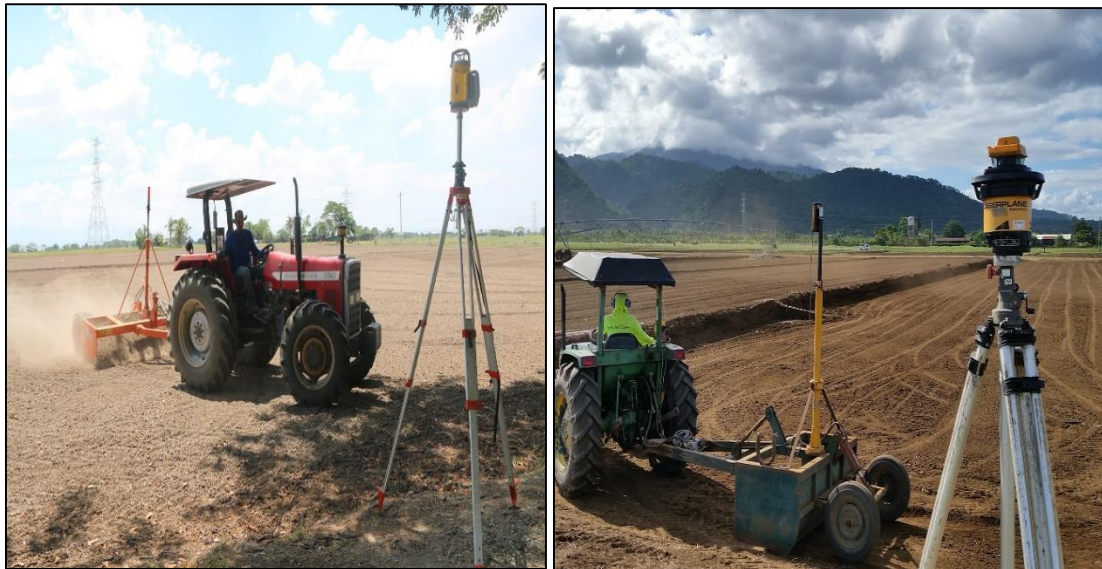
Fig 2 & 3: Laser Land Levelling at International Rice Research Institute (IRRI), Philippines.
