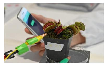
The team induced the Venus flytrap for closing its leaves in 1.3 seconds on demand by using the smartphone for transmitting the electric pulses to device at a specific frequency (Wenlong Li *et. al.*, 2021).
