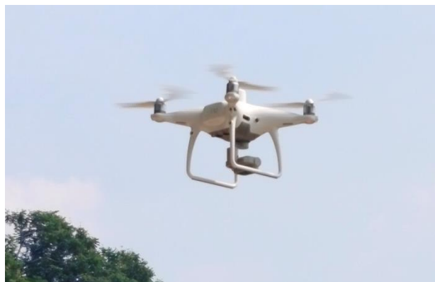
Fig.2 Multispectral imaging drone (DJI Phantom 4)
