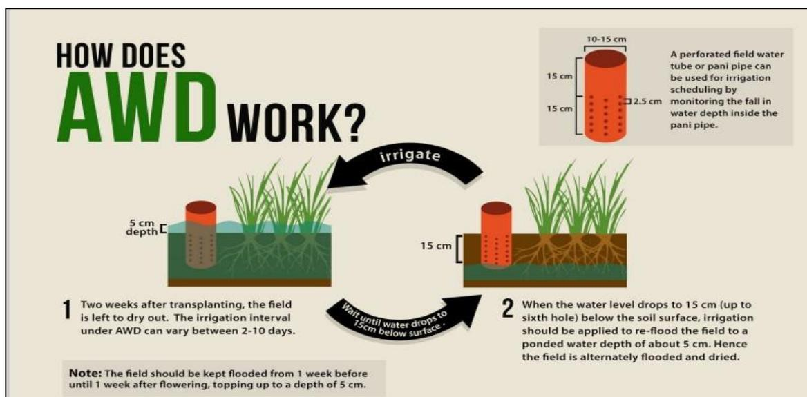
**Fig. 1:** Working principle of AWD technique
