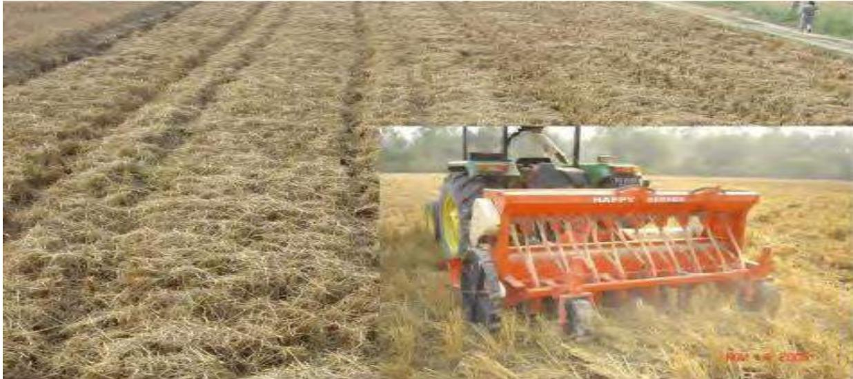
**Fig 5. Happy seeder sowing wheat into rice residue after uniform distribution of residue**
