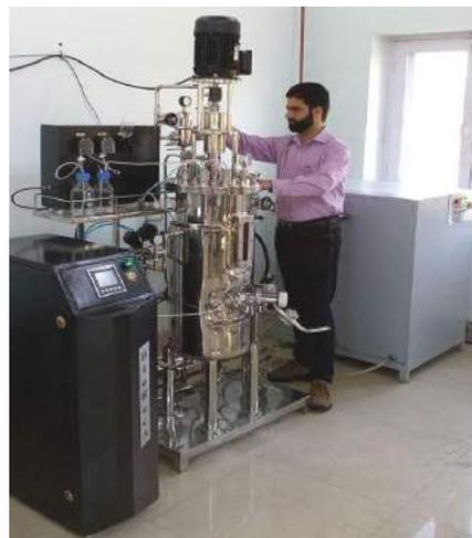
Fig.8. Fermenters for mass scale production of biofertilizers
