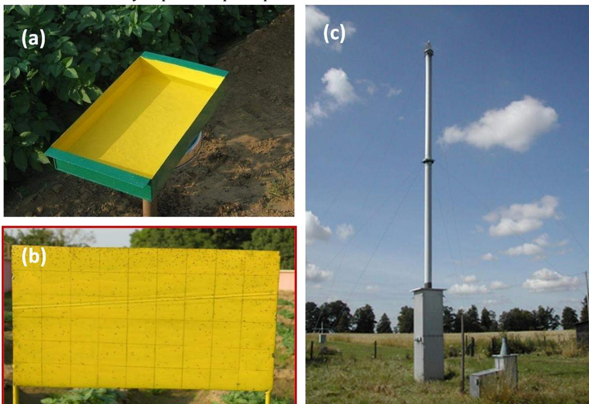
Fig. 1.1: Common aphid sampling methods: (a) yellow water pan trap; (b) yellow sticky trap; (c) suction trap (courtesy of Rothamsted Research).
