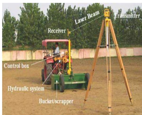
Fig.1 Laser leveler and its components
